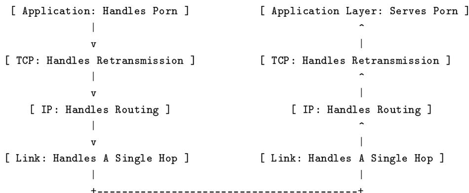
So in the diagram, we see Netscape (the Application on top left) retrieving a web page from a web server (the Application on top right). To do this it will use 'Transmission Control Protocol' or 'TCP': over 90% of the Internet traffic today is TCP, as it is used for Web and EMail.
